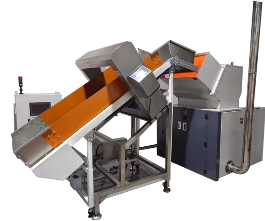
Connection to the plant's pneumatic conveying system
